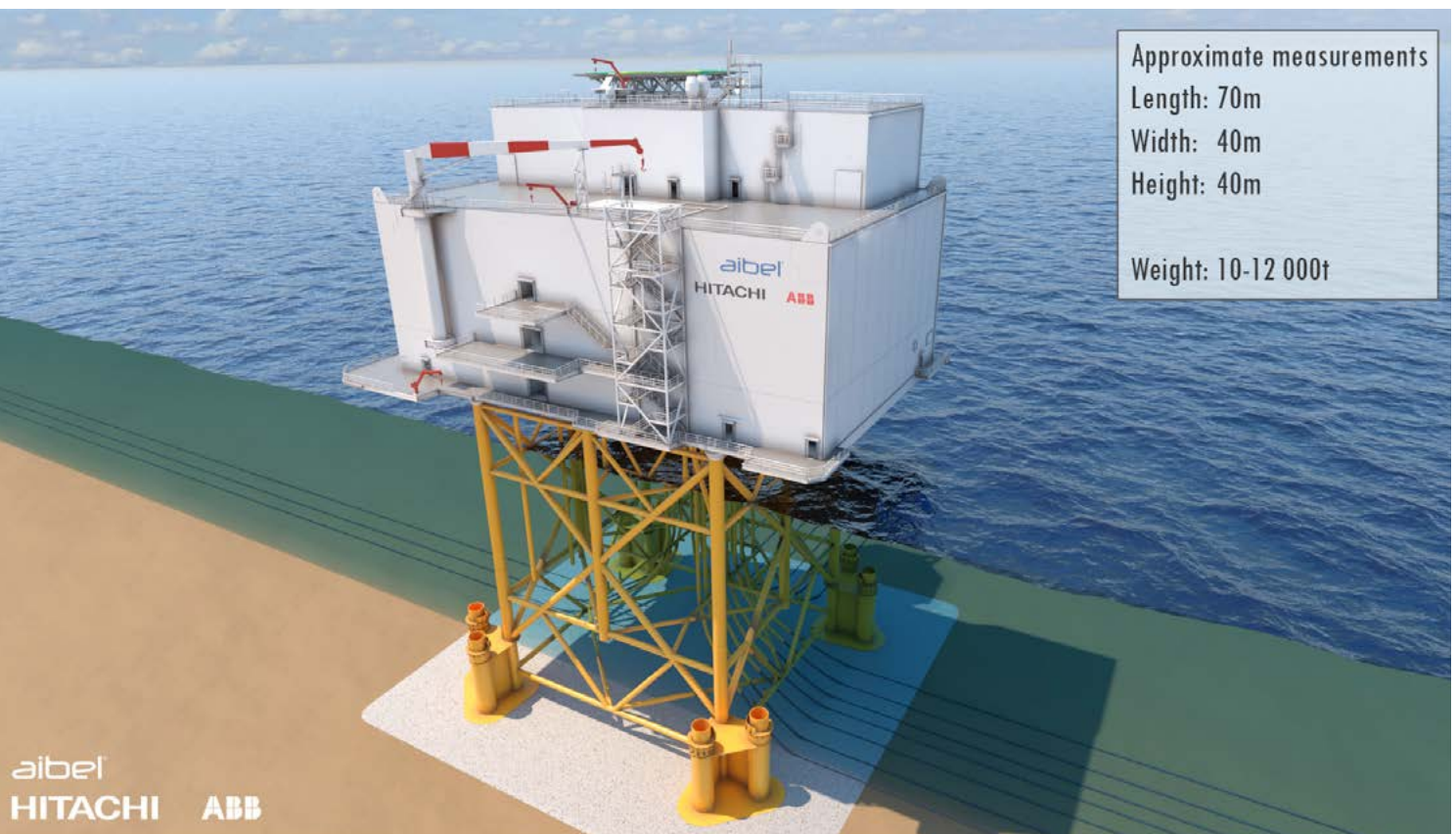
HVDC Converter Station. Photo: Aibel
