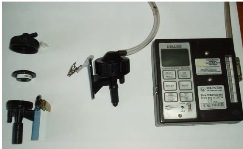
Figure 3. Sampling equipment. A dismantled cyclone is shown at the left of the picture, with a test cassette and filter in the centre. At the right is shown an assembled cyclone with a tube connected to the cyclone's inlet and a tube connected to the dust pump's inlet.
